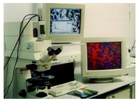
The new Zeiss Confocal Laser Scanning Microscope (CLSM)
