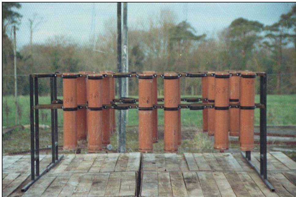
Plate 3. One replicate of intact soil/water columns mounted on holding rack.
