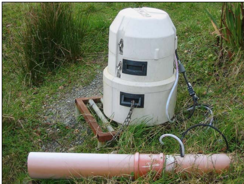
Plate 1. Portable water sampler with interfaced velocity probe and intake sampling tube at wetland inlet one monitoring station.
