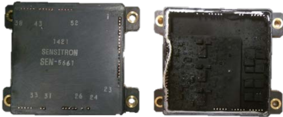
Figure 20: Three-phase bridge rectifier (left), after removal of top plate (right). Both top views.
