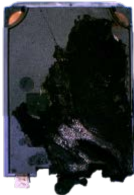
Figure 23: IGBT removed from bridge rectifier with melted wire bonds.
