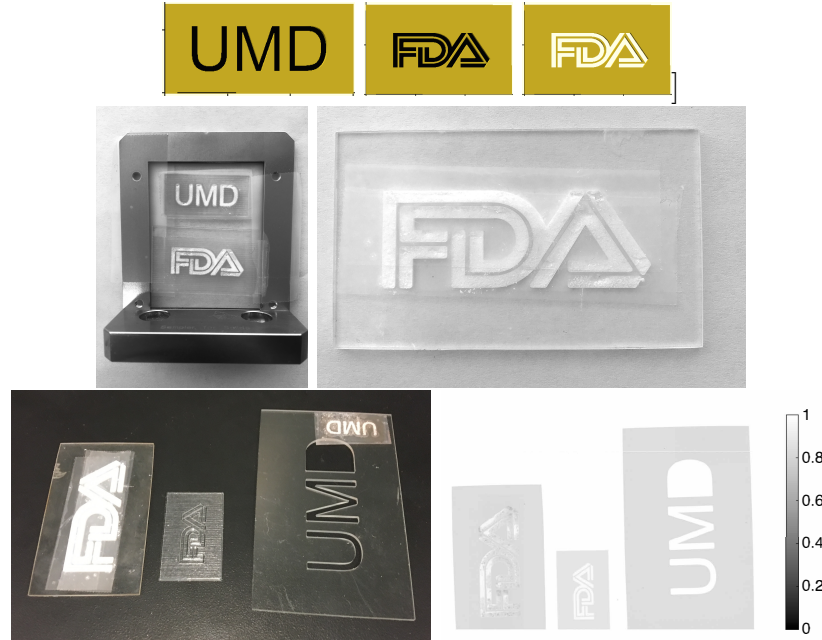
Figure 5.5: (Top row) OpenSCAD visualization of the phantom geometries. The first two were designs for the 3D printer with support material. The last was used as a stencil for CNC milling. (Middle) Photograph of 3D-printed Veroclear phantoms attached to sample holder and of the CNC-milled PMMA. UMD was 3.00x1.50x0.11 cm and FDA was 4.0x2.5x0.11 cm in size. The lettering and logo regions dipped inward and had a thickness at the bottom of the well of 0.01 cm. (Bottom right) Photograph of CNC-milled PMMA with dimensions 7.00x4.60x0.12 cm. The FDA logo was cut all the way through. (Bottom) Photograph of the phantoms imaged in absorption mode and absorption x-ray images of phantoms.
