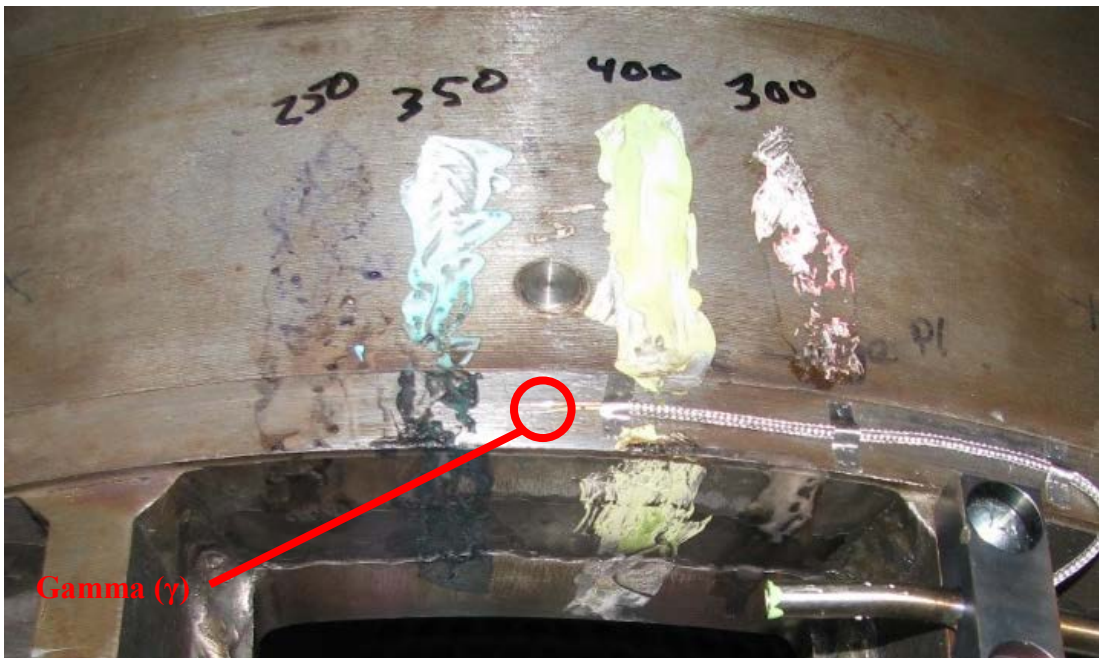
Figure 3.6: Temperature Melting Paint after Test Program
