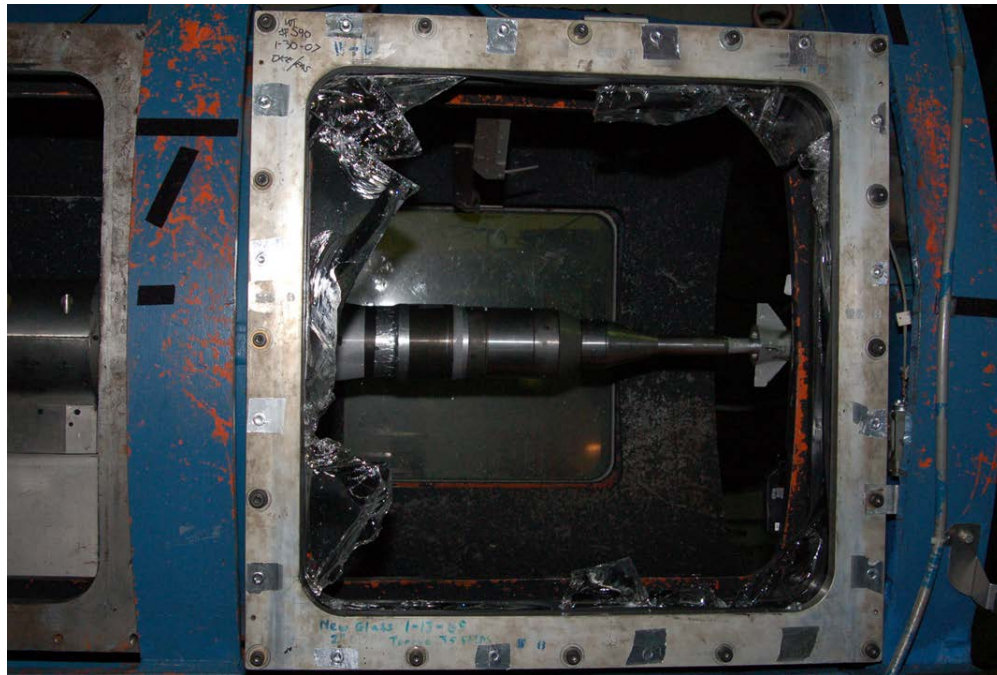
Figure 1.3: Broken Test Cell Window
