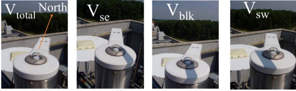
Figure 2.1. Four-step measurement cycle of the MFRSR instrument.
