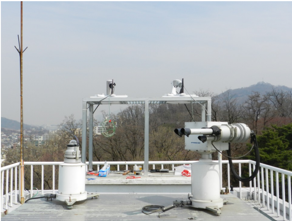
Figure 5.2. Instrumentation at Yonsei University in Seoul, South Korea. Top-left: UV-MFRSR, top-right: VIS-MFRSR, bottom-left: Skyview, and bottom-right: SKYNET Skyradiometer.
