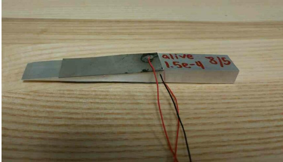
Figure 2.6: Image of a bimorph piezoelectric actuator.
