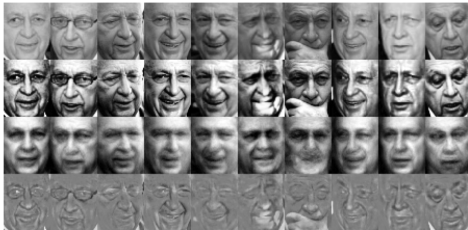
Figure 3.9: A subset of images from FIW(10b) demonstrates the low-rank decomposition of feature matrix in MCar: the original face images, histogram-equalized images \mathbf{X} , low-rank component \mathbf{Z} , and noisy component \mathbf{E}_X , from the first row to the fourth row, respectively.
