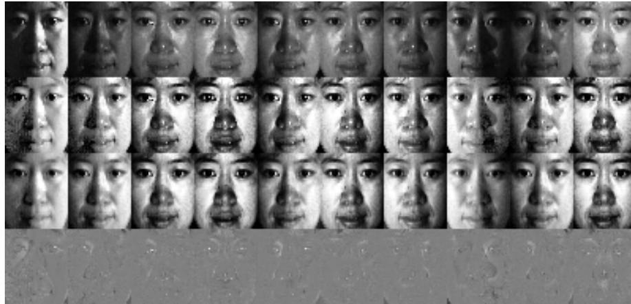
Figure 3.10: A subset of images from the CMU PIE dataset demonstrates the low-rank decomposition of feature matrix in MCar: the original face images, histogram-equalized images \mathbf{X} , low-rank component \mathbf{Z} , and noisy component \mathbf{E}_X , from the first row to the forth row, respectively.
