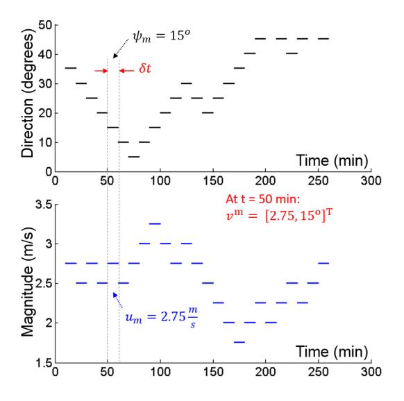
Figure 5.2: Model of the flowing medium.
