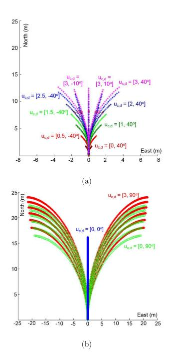
**Figure 3.8:** (a) A dynamically feasible control action set  $\mathcal{U}_{c,d}$ , and (b) a dynamically feasible contingency control action set  $\mathcal{U}_{e,d}$  for the USV14 with different initial surge speeds.
