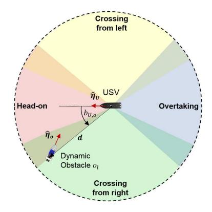
Figure 3.2: COLREGs head-on, crossing from right, and overtaking behaviors.
