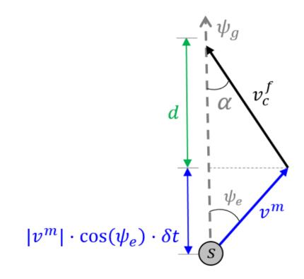
Figure 5.5: Calculation of additional compensation cost-to-go for free-flowing action  $\mathbf{u}_{f,d}(\mathbf{s})$ .
