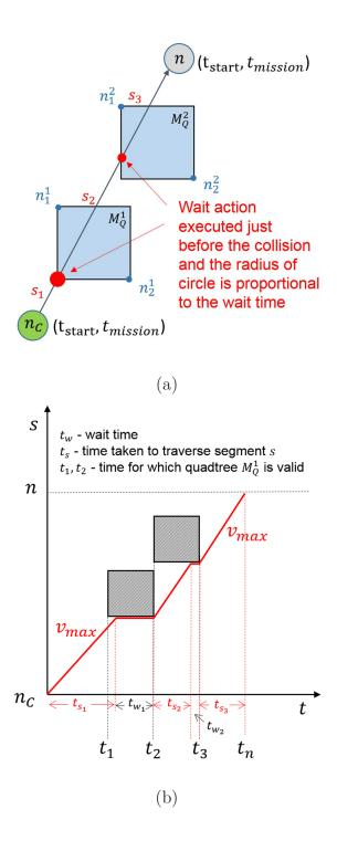
Figure 4.17: (a)Example illustrating the computation of travel cost from the current node  $\mathbf{n_c}$  to node  $\mathbf{n}$  in an environment with two quadtrees  $\mathcal{M}_Q^1$  and  $\mathcal{M}_Q^2$ .(b) Graph of time v/s distance shows the progression of the computed path with traversal time for each segment denoted by  $t_s$  and wait time by  $t_w$
