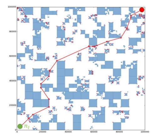
Figure 4.22: Experimental setup and sample any-angle path from the start node  $n_I$  to the goal node  $n_G$ .
