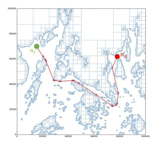
Figure 4.24: Computed path on a real world scenario.
