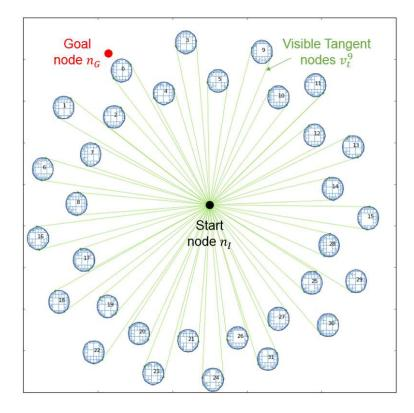
**Figure 4.8:** Pathological scenario where a node in tangent graph has a large branching factor.
