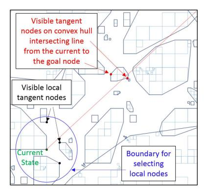
Figure 4.9: Procedure to add nodes to the focused visibility graph.
