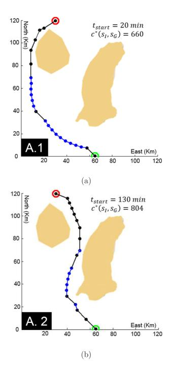
**Figure 5.6:** Comparison of paths for the scenario A with different start times. The green circle represents the initial location and the red circle represents the goal location of the vehicle. Each blue segment is a free-flow action and each black segment is a thrust-producing action.
