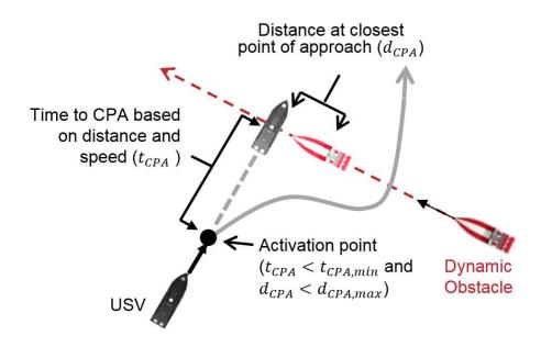
Figure 3.3: Calculation of CPA time and CPA distance.
