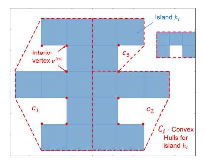
Figure 4.4: Eliminating visible interior vertices from the visibility graph (.
