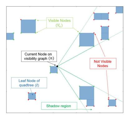
Figure 4.3: Computation of visible nodes in quadtree.
