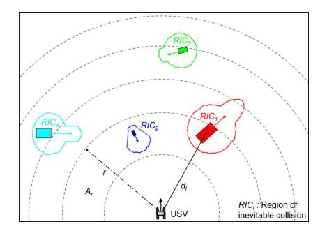
Figure 3.9: Computation of the congestion metric for an example scenario.
