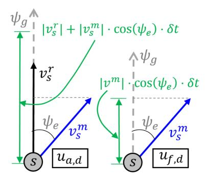
Figure 5.4: Calculation of heuristic #2.
