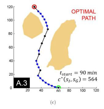
**Figure 5.6:** Comparison of paths for the scenario A with different start times. The green circle represents the initial location and the red circle represents the goal location of the vehicle. Each blue segment is a free-flow action and each black segment is a thrust-producing action.
