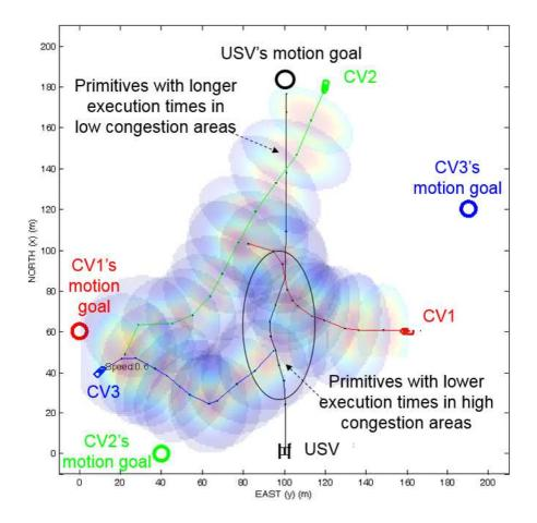
**Figure 3.5:** An example of a computed risk and contingency-aware, dynamically feasible trajectory using adaptive control action primitives in a scenario with 3 civilian vessels
