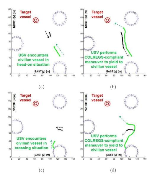
**Figure 3.10:** The experimental results of the USV14 autonomously dealing with "head-on" (see a) and b)), "crossing from right" (see c) and d)), and "overtaking" (see e) and f)) situations
