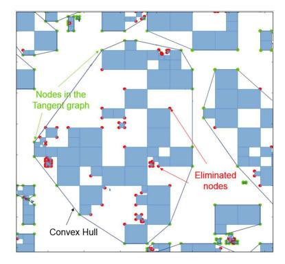
Figure 4.5: Eliminating nodes in the interior of the convex hull (we assume the start and the goal node are not inside any convex hull)
