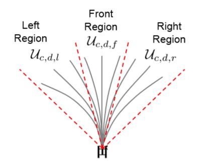
Figure 3.4: A set of control action primitives divided into three sub-regions.
