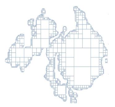
Figure 4.2: Quadtree representation of a complex polygon.
