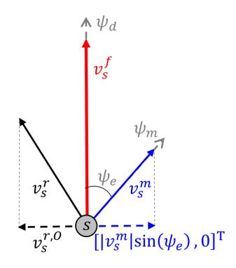
Figure 5.3: Computation of vehicle's forward velocity under medium flow.
