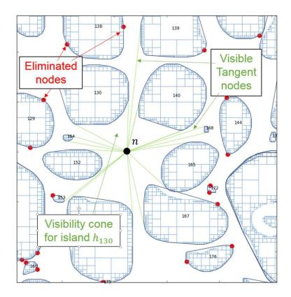
Figure 4.6: Elimination of non-visible nodes using the computed tangents for the islands in H
