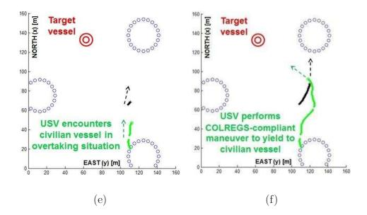
**Figure 3.10:** The experimental results of the USV14 autonomously dealing with "head-on" (see a) and b)), "crossing from right" (see c) and d)), and "overtaking" (see e) and f)) situations
