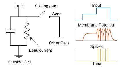
Figure 1.2: **LIF neuron as a circuit** *Left:* Circuit diagram. *Right:* Neuron behavior.
