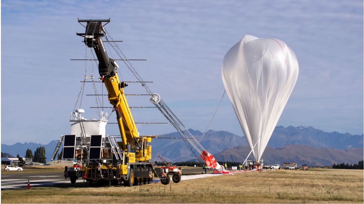
FIGURE III.6: Picture of a balloon launch. The payload is captured by the launch vehicle (in yellow) until the balloon is inflated and released. The parachute assembly, which is a part of the long train from the top of the payload to the bottom of the balloon, can be seen in red. Credit: NASA.
