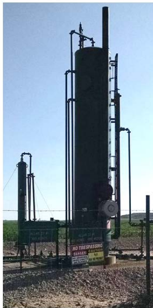
Fig. 3-1. Battery separation column
