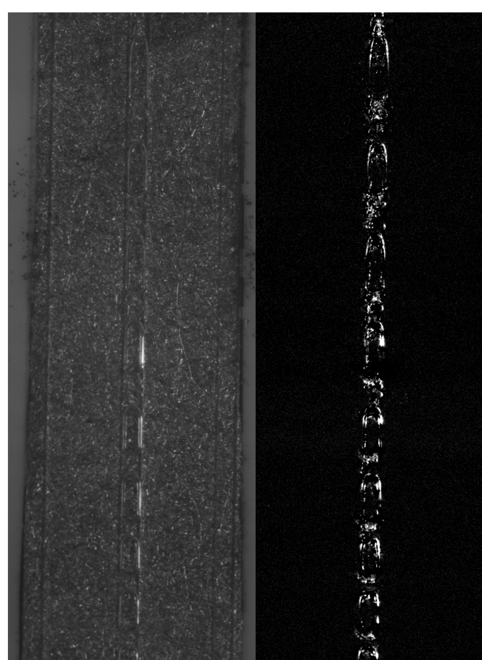
Fig. 5: Taylor flow in the outlet channel. (Current density=2, St.No.=100)
