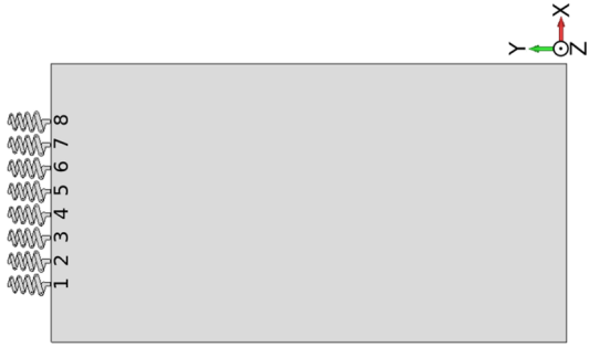
Figure 2. Phased antenna array configuration on the ground plane.
