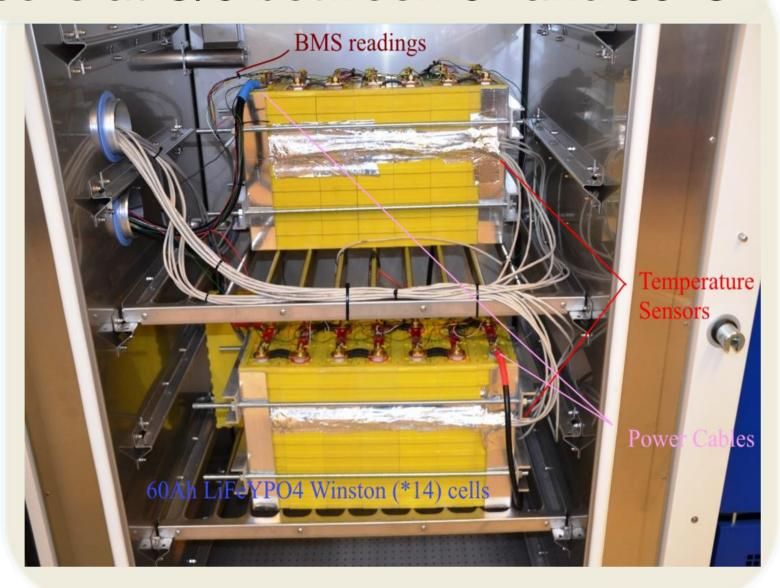
14\*CALB 60Ah LiFePo4 cells at C/5 and C/10 charge current rate
