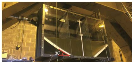
Figure 7: TLD with sloped bottom of an angle of 30°
