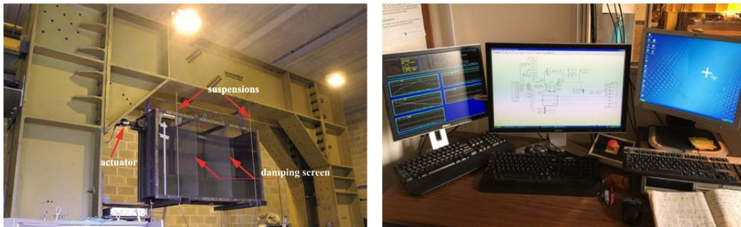
Figure 3: Test setup. (a) the reaction frame and the physical substructure (the TLD). (b) control room
