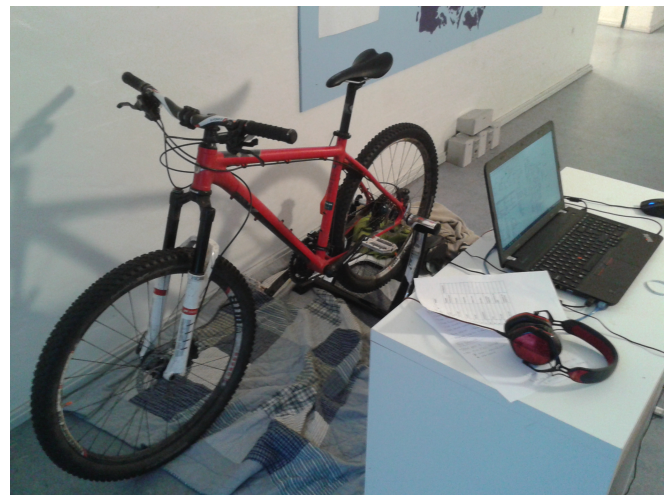
Figure 3. Illustration of the test setup. The blankets were used in an attempt to reduce vibrations and noise.
