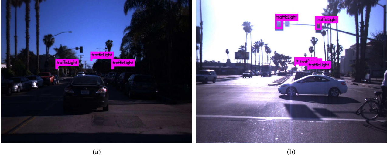
Figure 6: Results from YOLO V3 1 applied on LISA-daySeq1.
