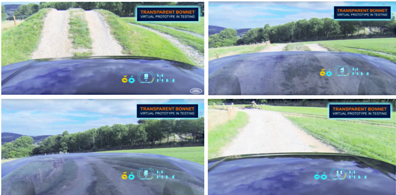
Figure 2: The vision video of ‘The Transparent Bonnet system’ showing the SUV approaching a hill, prompting the augmented reality (AR) HUD to make the front hood semi transparent while climbing the hill, before it again turns solid (Land Rover UK 2014a).
