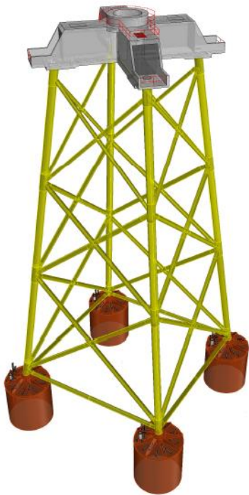
Siemens Jacket concept for +10 MW wind turbine.
