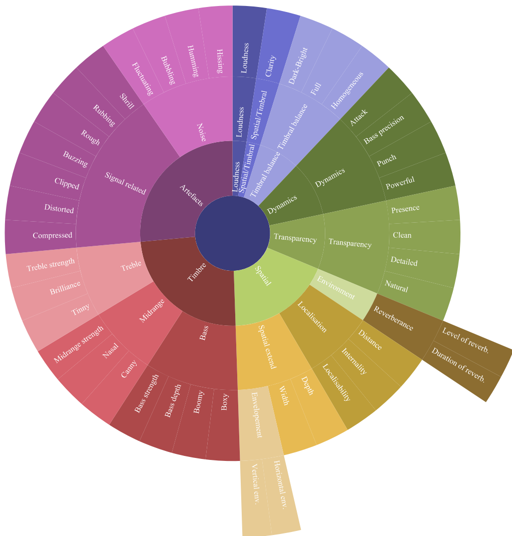
Fig. 5: Sound wheel of sensory descriptors for perceptual characterisation of reproduced audio. The rings (in→out) represents, groups, subgroups, and sensory descriptors respectively. Adapted from [66, 84] and generated using an Aculocity visualization tool ( www.aculocity.com/labs/sunburst-chart ).
