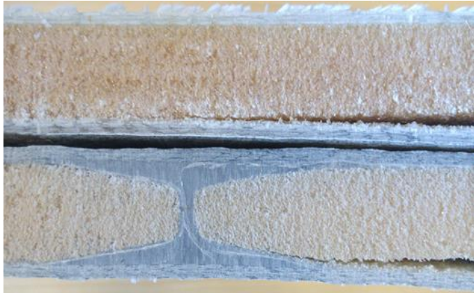
Figure 45. Post mortem sections of sandwich panel specimens PLT2 (above – no peel stopper) and PLP2 (below - with embedded peel stopper), [56].
