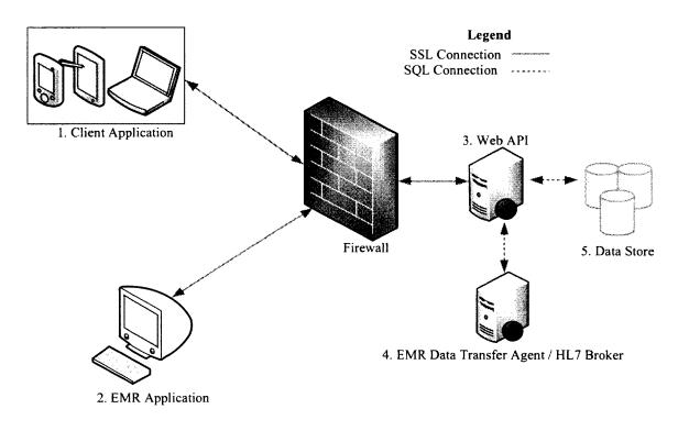
Figure 3.3 Secure Data Sharing Architecture (SDSA)
