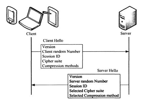
Figure 3.1.2 Establishing Security Capabilities [15]
