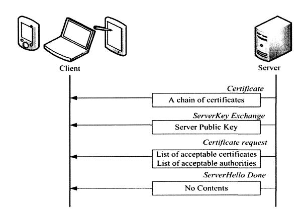
Figure 3.1.3 Server Authentication and Key Exchange [15]
