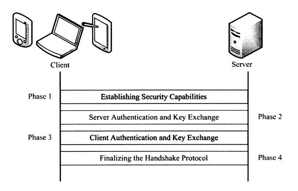
Figure 3.1.1 SSL Handshake Protocol [15]
