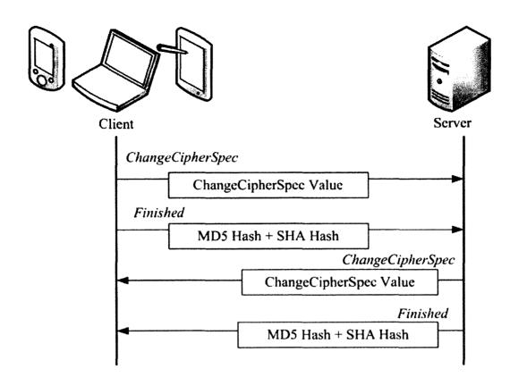
Figure 3.1.5 Finalizing the Handshake Protocol [15]
