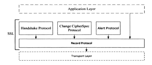
Figure 3.1 SSL Protocol Stack [15]
