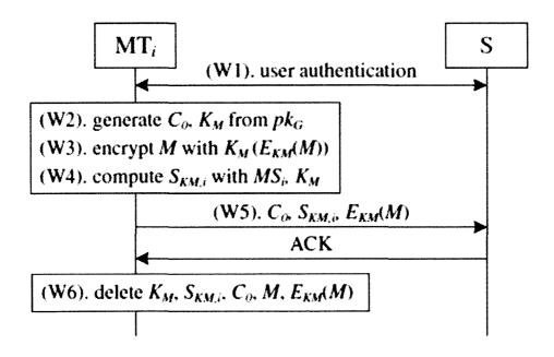
Figure 2.4.2 Write Process [20]
