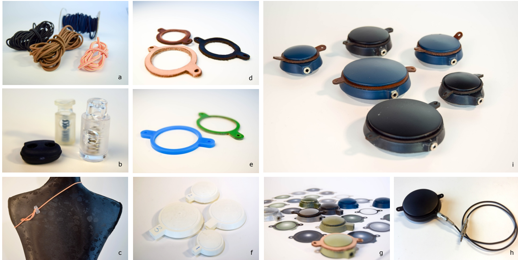
Figure 11. Explorations of materializations of the vibrating domes for the Hedonic Haptic player. Previous experiments showed that the placement and adjustment of the encased motors should be flexible and that the motors had to be fastened with a relatively tight fit to enable the best sensations of the vibrations. We explored elastic strap-on mechanisms and found that a round elastic band (a) in combination with cord lock (b) would be a least intrusive solution (c). To attach the vibrating domes to the elastic band some tolerance was needed, as the motion of a moving body would cause dispositions of statically attached vibrating elements. A ring shaped mechanism that could be pulled over the vibrating domes would provide some rotation freedom. We then explored leather materials (d), and Perspex and rubber materials (e) to find the right stretch, tolerance, and aesthetic of these rings. Different dimensions of the domes were explored (f), as well as a color scheme close to the Beoplay look (g). This resulted in one all black version of the Hedonic Haptic player with black leather and elastic band, and one in dark petroleum with brown leather and elastic band (i), with metal details in the cable (h). Here, materializing the domes dynamically worked together with experiencing physical form elements.
