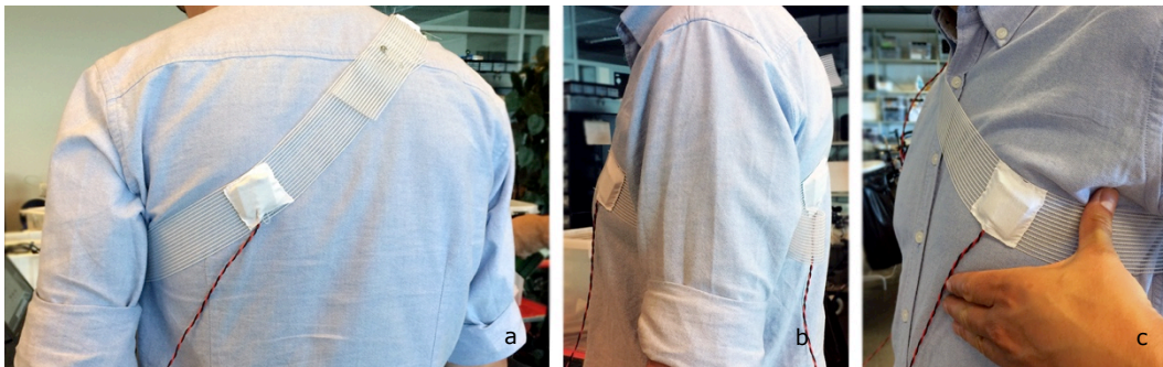
Figure 4. The rubbers were mounted in cotton patches and attached to elastic band to explore vibrations on different places on the body (a,b,c).
