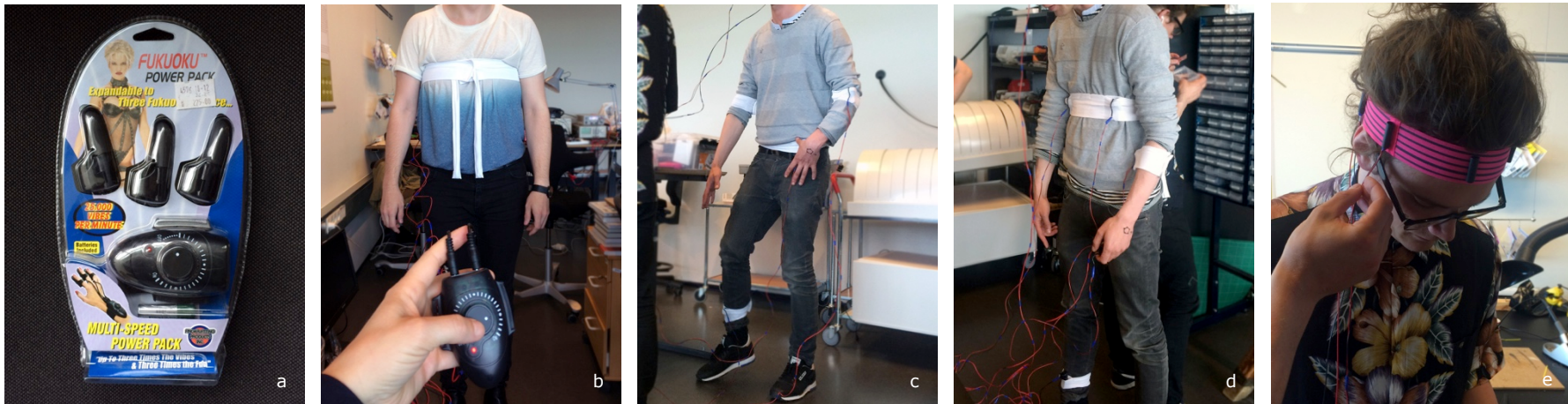
Figure 2. Experiments with modified off-the-shelf vibrators from a sex shop (a) embedded in elastic and cotton bands. The vibrating sensations were explored on different parts of the body, among others the chest (b), the ankles and elbows (c), the forearms and the diaphragm (d), and head (e).
