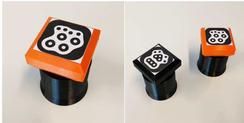
Figure 9: Environment objects. Items to be placed in the environment for the robot to interact with. They are light enough to be pushed yet stable and will not fall over easily. The tool connector with fiducial is mounted on top.
