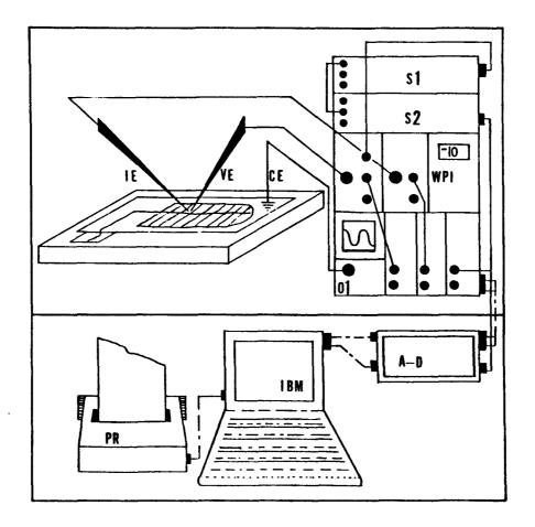
The current injected was linear with the voltage applied to the external input in the S-7050A module; it was monitored on oscilloscope (01). The second trace, the electrotonic potential trace, was recorded by the APL acquisition and analysis programs. Current tracings were not stored. The RMP of the cell was monitored by the penrecorder.
