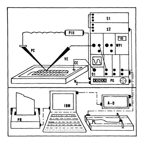
potential. A variety of ACh-containing electrodes were tried, as well as, two different means of injection: an iontophoretic unit and two Grass S-88s were used for retention and ejection currents.
