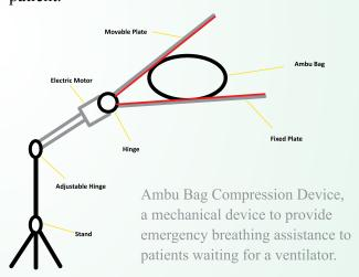
To deal with this painful situation, we designed a device, Ambu Bag Compression Device (ABCD) to replace the human hand with a mechanical device. It has automated rate and pressure control according to the age of child. Such a device can reduce mortality and morbidity while also reducing parents' anxiety and stress. This can be manufactured locally with local expertise and can be mass produced.
