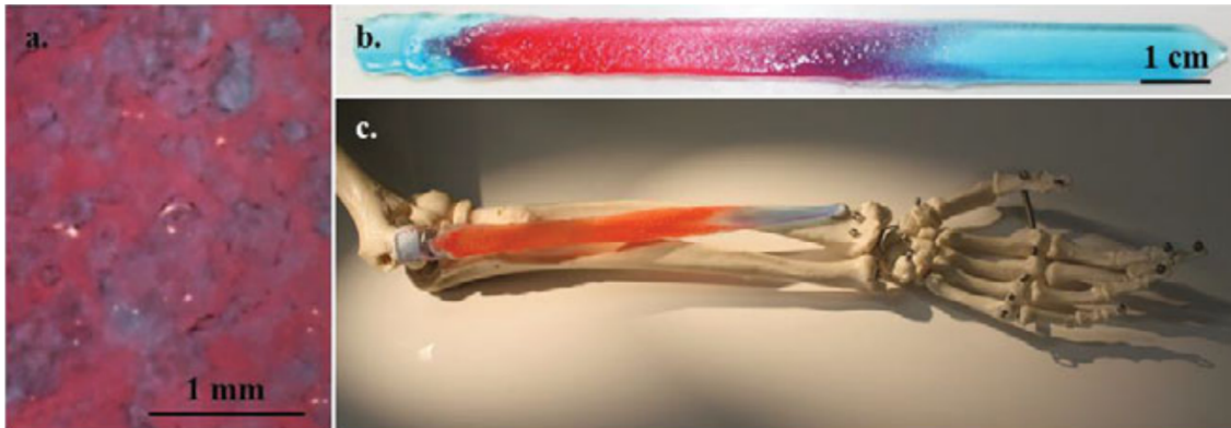
Figure A.8: (a.) Macroscopic image of a 3D printed particulate reinforced Alg/p-AAm ICE gel composite ribbon with an Emax volume fraction of 40 %. (b.) Photograph of an artificial tendon printed with Alg/p-AAm ICE gel and Emax gradient structures. (c.) Photograph of a 3D printed artificial tendon attached to a skeleton.
