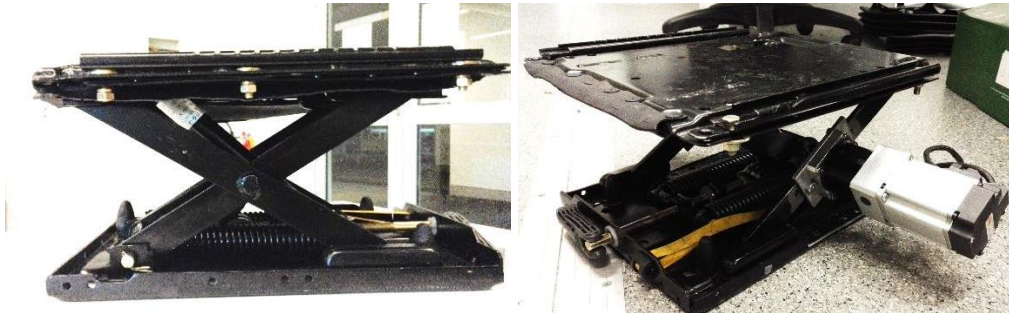
Fig. 3. Conventional passive seat suspension and active seat suspension prototype
