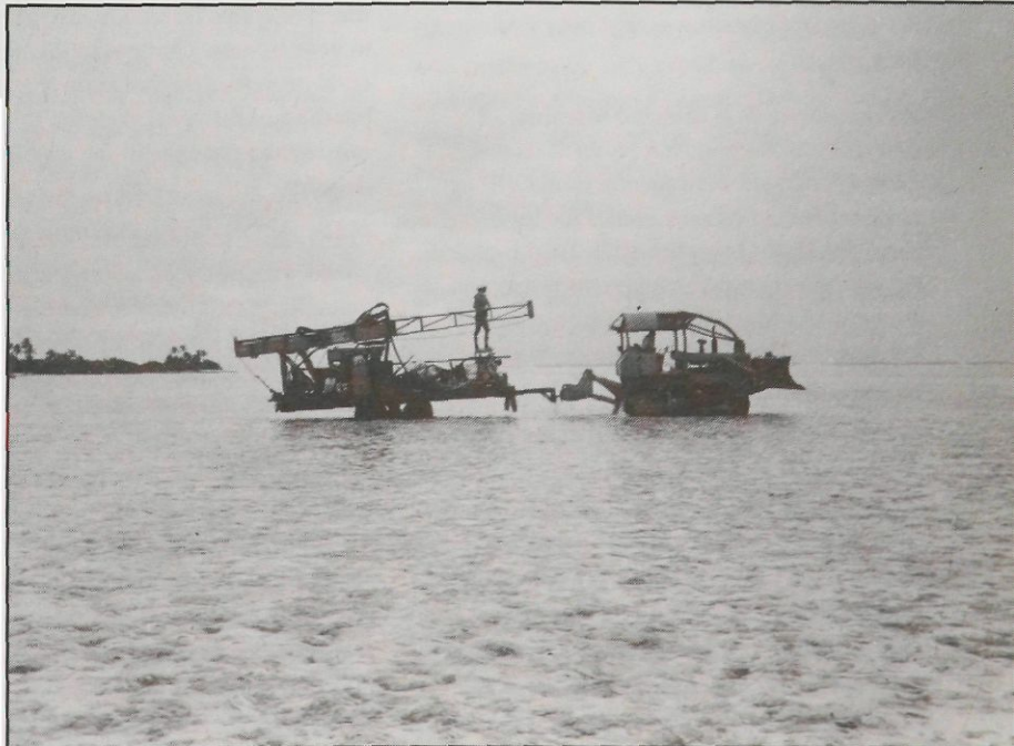
Transporting a drilling rig across the reef at low tide on Cocos (Keeling) Islands to reach the least accessible islands
