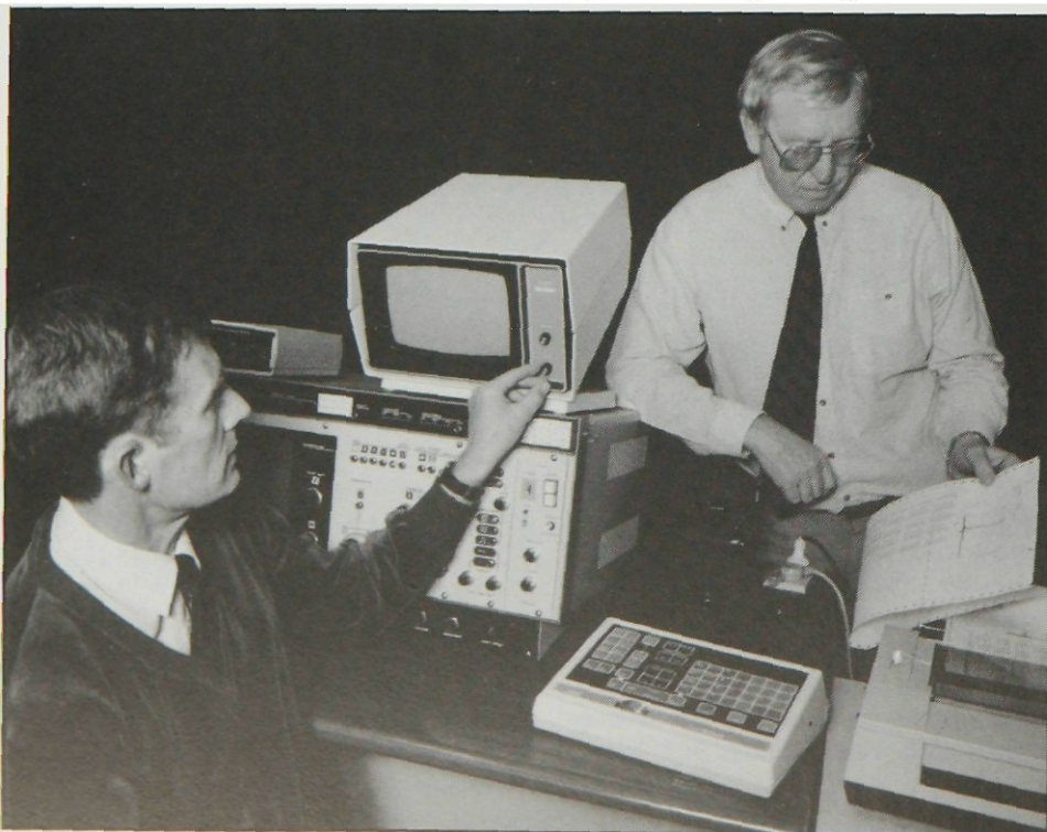
Associate Professor Druce Dunne and Dr Gordon Delamore examine an alloy compositional analysis obtained from an x-ray energy dispersive spectrometer attached to a Hitachi Scanning Electron Microscope in the Department of Materials Engineering
