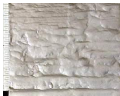
Fig. 3. The defects of slab billet [3]
