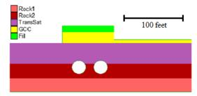
Figure 2. FLAC model: geological strata + tunnels
