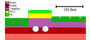
Figure 3. FLAC model: geological strata + tunnels + applied loads
