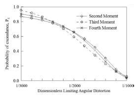
Figure 5. Probability of exceedance at various levels of limiting angular distortion for building 1
