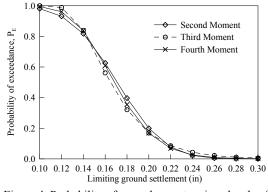
Figure 4. Probability of exceedance at various levels of limiting ground settlement
