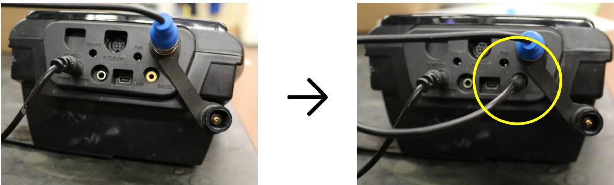
Figure 30. Connecting the USB to RS232 to the Orion Star pH meter.
