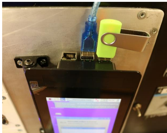
Figure 32. Complete USB RPI connections.
