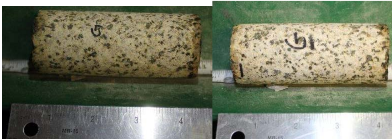
Figure 54: Sample G prior to axial load. No distinct cracks present in core.
