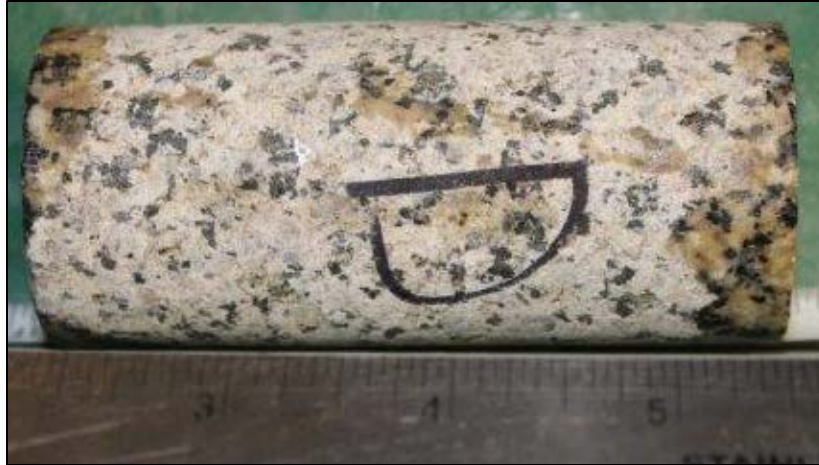
Figure 73: Sample D after triaxial load. Sample failed nonviolently, no distinct shear planes present.
