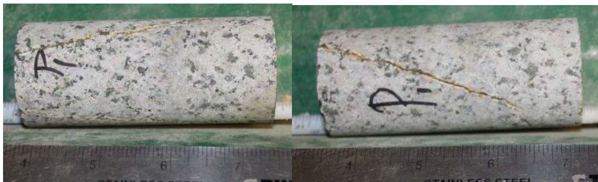
Figure 67: Sample P1 prior to axial load. Large crack approximately 30° from vertical.
