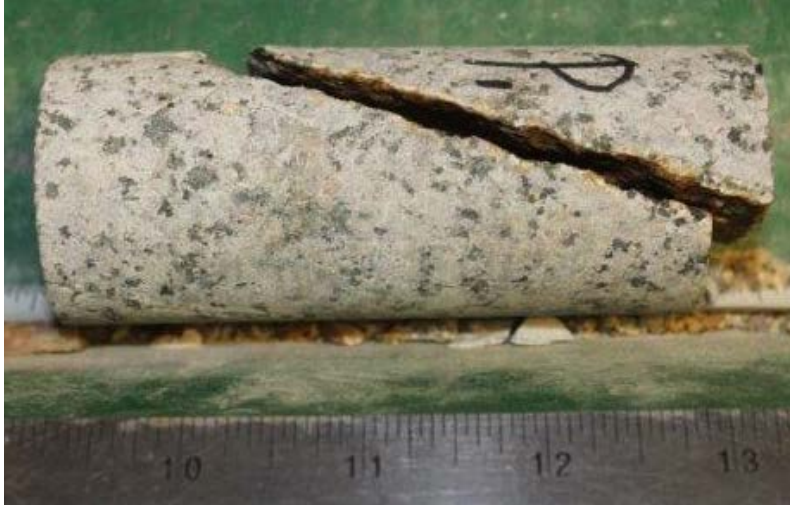
Figure 68: Sample P1 after axial load. Sample compressed until brittle failure occurred along major discontinuity.
