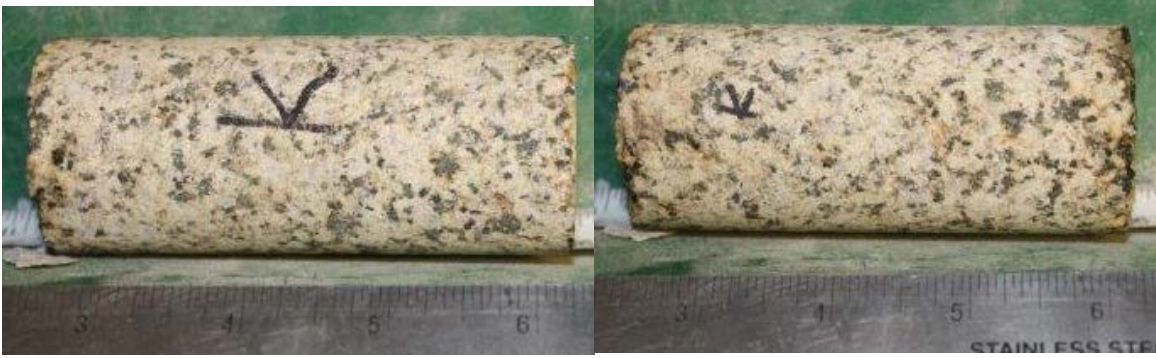
Figure 58: Sample K prior to axial load. No distinct cracks present in core.
