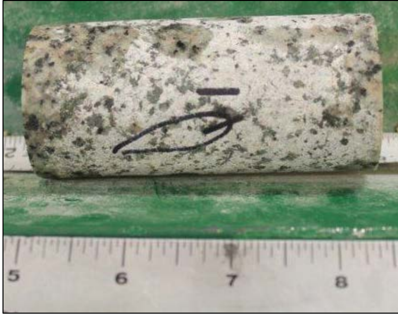
Figure 84: Sample Q1 after triaxial load. Sample failed nonviolently. No shear fracture planes are visible.
