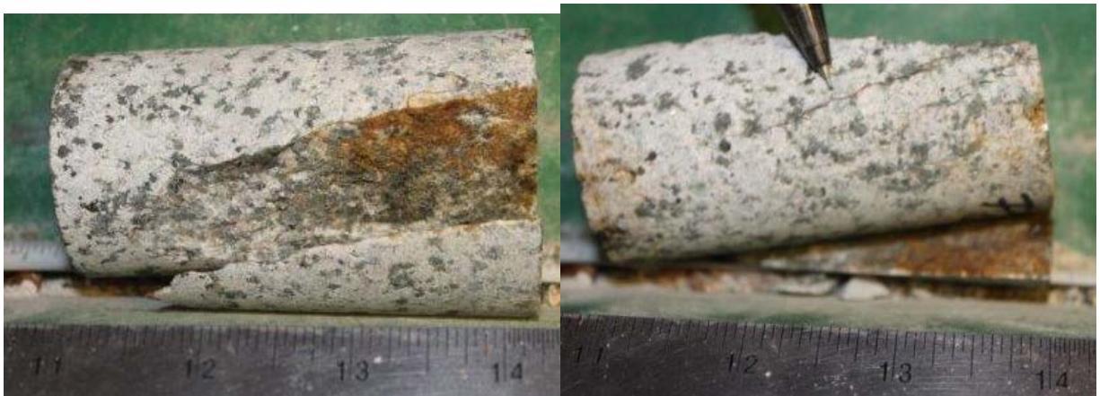
Figure 70: Sample P2 after axial load. Sample compressed until first brittle cracking occurred along major discontinuity, causing sharp drop in axial pressure. Failure occurred shortly after, causing additional cracking to form throughout the core sample.
