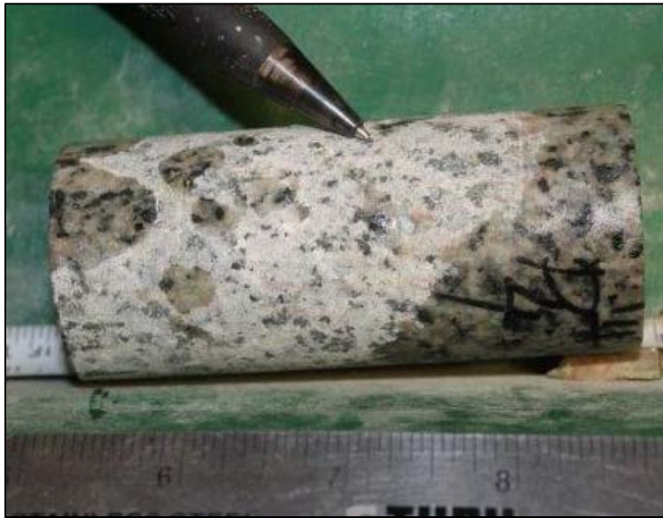
Figure 77: Sample P4 after triaxial load. Sample failed nonviolently. Small shear fracture indicated with pencil.
