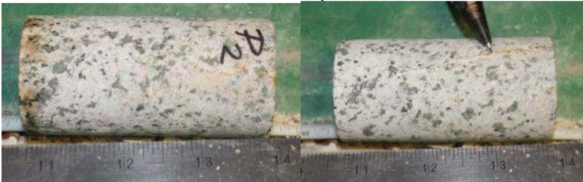
Figure 69: Sample P2 prior to axial load. Small fracture indicated with pencil.
