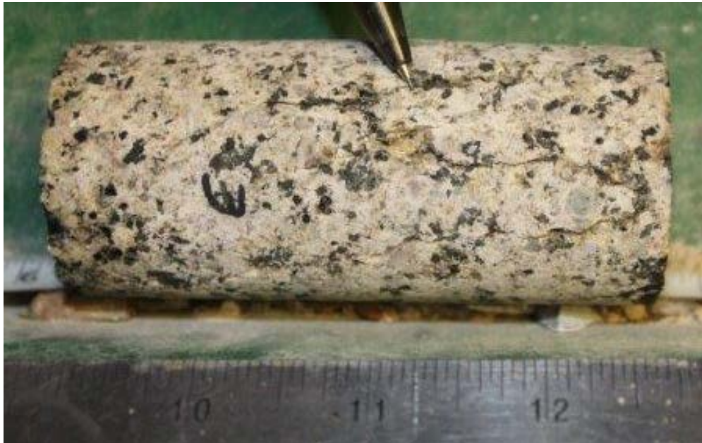
Figure 65: Sample E after axial load. No photograph was taken prior to axial load. Sample compressed until nonviolent failure occurred. Multiple axial splits developed while under load. Failure crack indicated with pencil.
