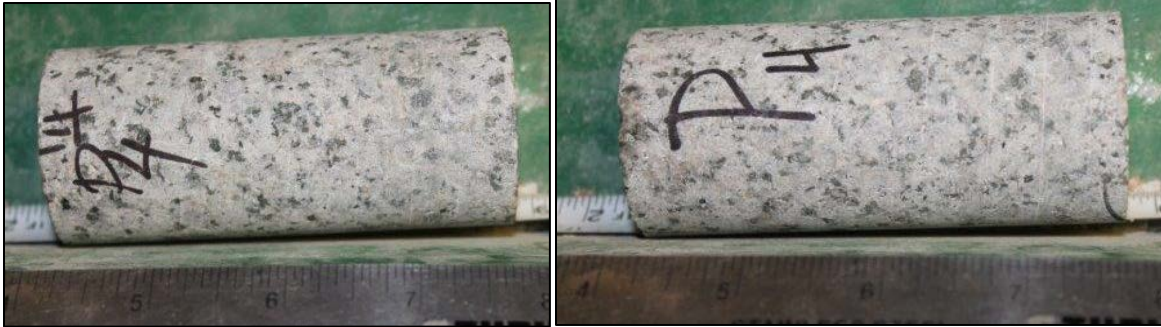
Figure 76: Sample P4 prior to triaxial load. No distinct cracks present in core.
