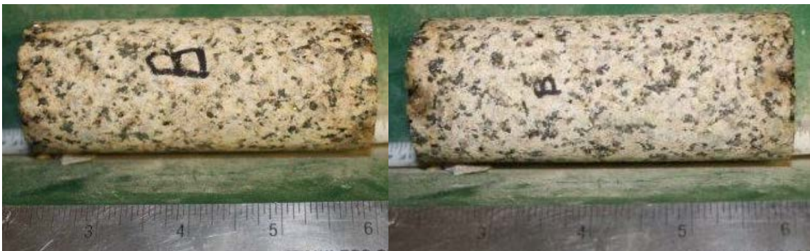
Figure 63: Sample B prior to axial load. No distinct cracks present in core.
