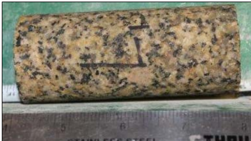
Figure 75: Sample L1 after triaxial load. Sample failed nonviolently, no distinct shear planes present.
