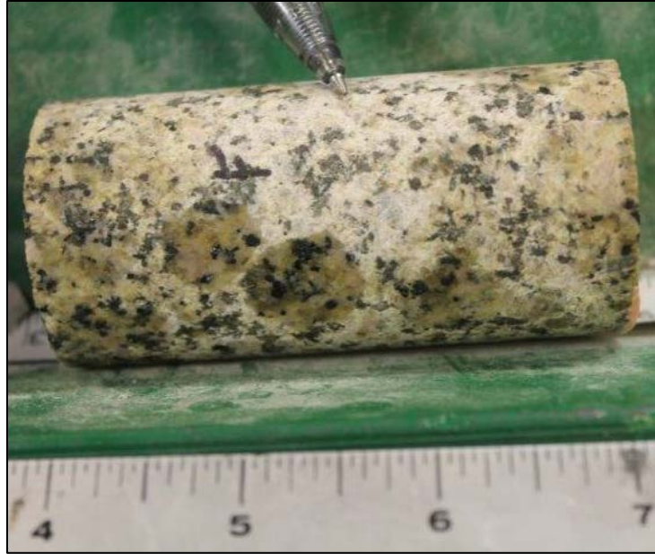
Figure 80: Sample F after triaxial load. Sample failed nonviolently. Small shear fracture indicated with pencil.
