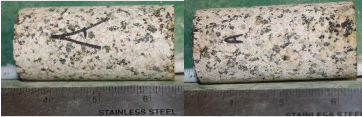
Figure 61: Sample A prior to axial load. No distinct cracks present in core.
