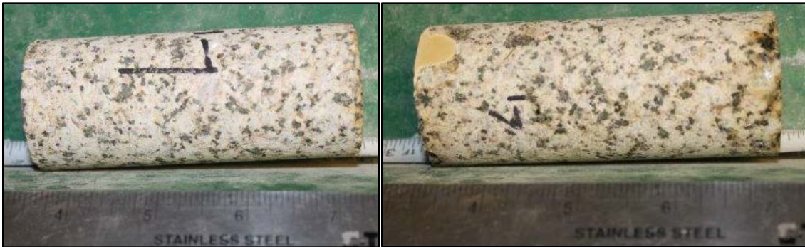
Figure 74: Sample L1 prior to triaxial load. No distinct cracks present in core. Small cracks patched with bolt anchor sulfaset yellow: high speed expansive anchoring compound.
