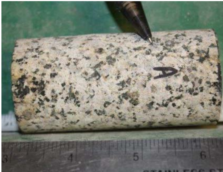
Figure 62: Sample A after axial load. Sample compressed until nonviolent failure occurred. Failure crack indicated with pencil.
