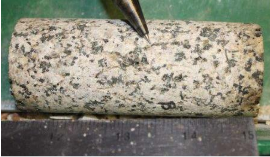
Figure 64: Sample B after axial load. Sample compressed until nonviolent failure occurred. Failure crack indicated with pencil.
