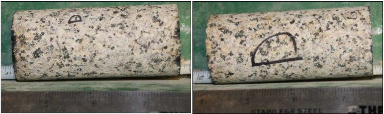
Figure 72: Sample D prior to triaxial load. No distinct cracks present in core.
