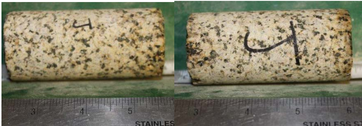
Figure 56: Sample J prior to axial load. No distinct cracks present in core.
