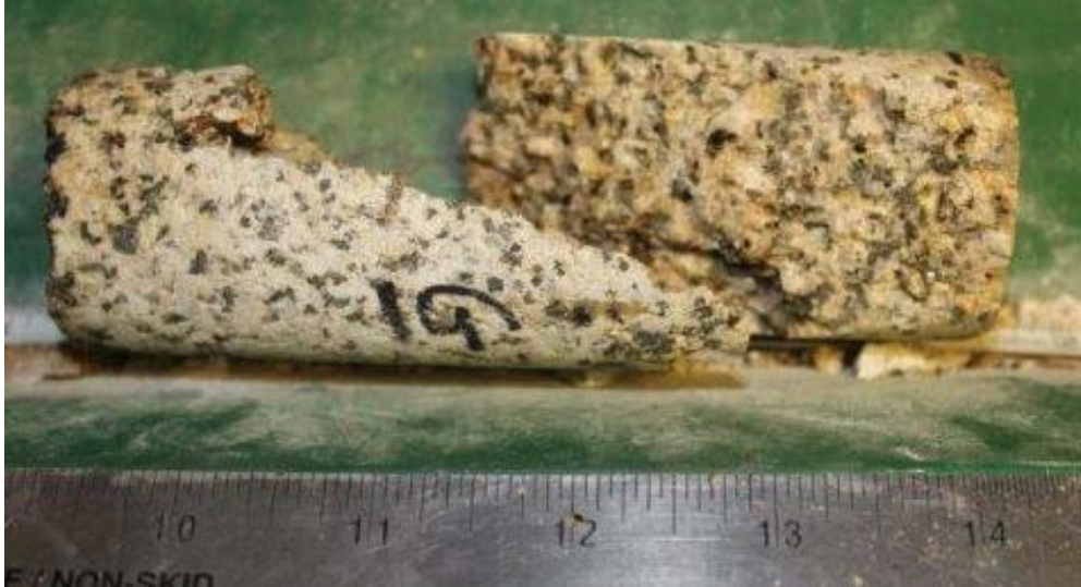
Figure 55: Sample G after axial load. Sample continuously compressed, causing force to undulate until nonviolent shear failure occurred.
