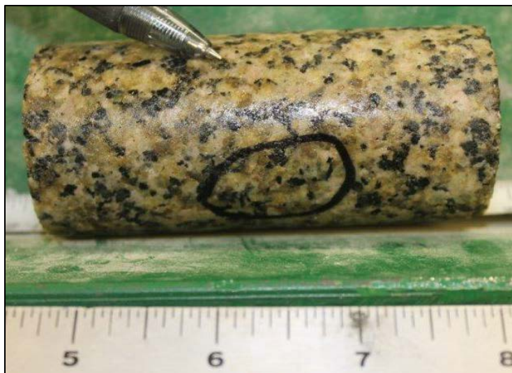
Figure 82: Sample O after triaxial load. Sample failed nonviolently. Small shear fracture indicated with pencil.
