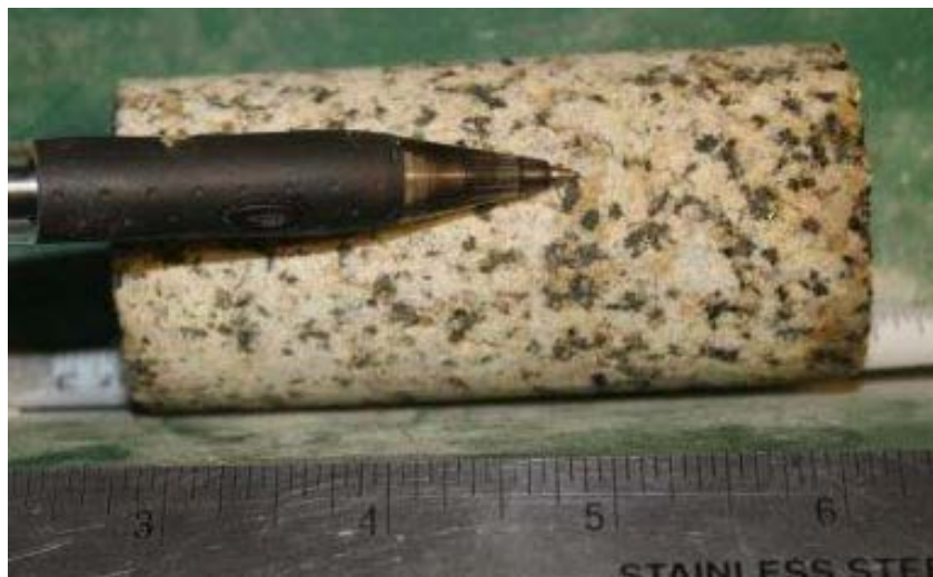
Figure 57: Sample J after axial load. Sample compressed until nonviolent failure occurred. Failure crack indicated with pencil.
