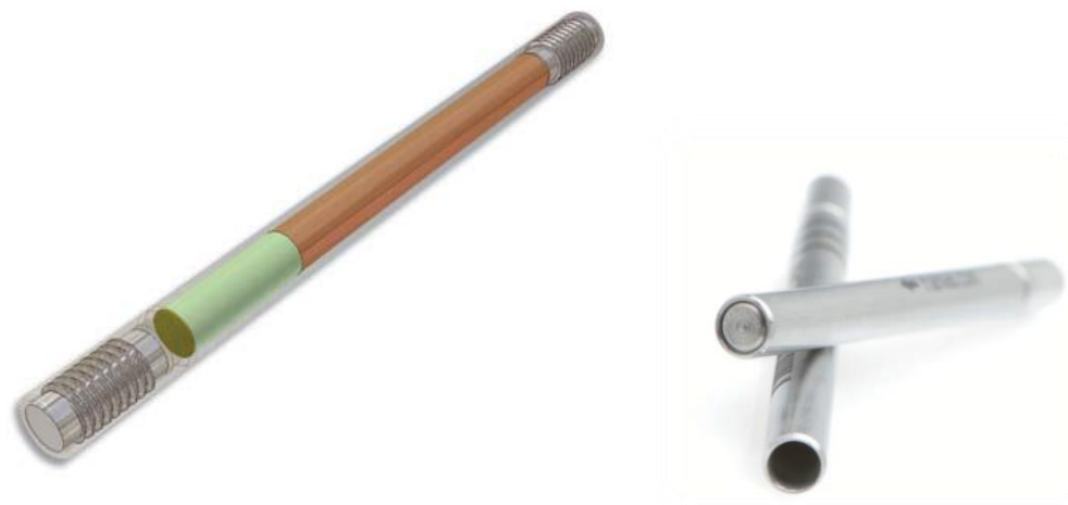
Figure 6. Schematic of SafeLok tube packed with two sorbents and a standard thermal desorption tube with and without SafeLok insert. 6
