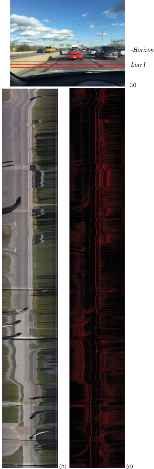
Figure 2 A road profile obtained from a sampling line at 10-15m ahead of vehicle. (a) An associated image region around the sampling line is also located for obtaining spatial property of road such as linearity of road edges. (b) The resulting road profile is displayed in right column. (c) The linearity is also displayed in red intensity. The horizontal axes are x and vertical axes are frame number t upward for both (b) and (c).
