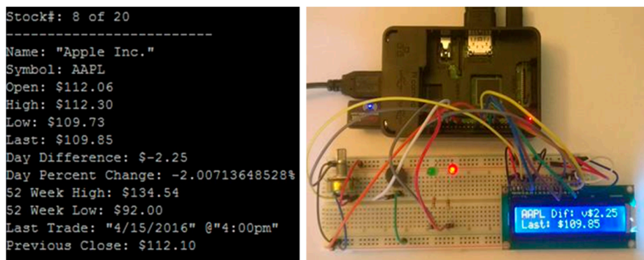
Figure 2. A prototype of the stock ticker system. The left side shows stock information in the terminal of Raspberry Pi. The right side shows the setup of the system: the stock information is displayed in the LCD, while the red LED indicates the price has dropped from the previous day's closing price.
