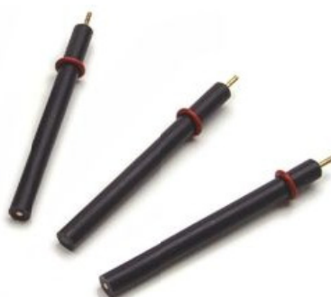
Figure 9 - Polycrystalline gold disk electrodes ( Au(111) ) provided from Bioanalytical Systems (area 0.020\text{ cm}^2 ) used as working electrode.
