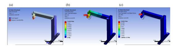
Fig. 6.4. Engineering Analysis of Stereotactic Device (a) Fixed support and Pressure location, (b) Deformation=1.2633 mm and (c) Stress=13.825 MPa
