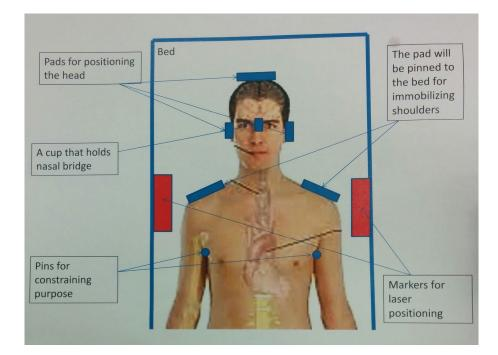
Fig. 5.10. Location of patient positioning and immobilization devices used in the new design
