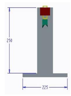
Fig. 5.32. Overall Dimensions of Stereotactic Frame
