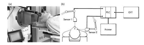
Fig. 2.1. (a) View of the patient motion monitoring system in the proton treatment room. The sensors are placed in AP and LAT direction. The OIT in the front displays the patient's motion data, (b) Schematic diagram of the patient motion monitoring system.
