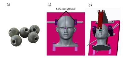
Fig. 5.4. Devices used for Tumor tracking in the new design (a) Spherical Markers, (b) Markers positioned in the new design, (c) Customized 3D printed nose bridge part(Green)
