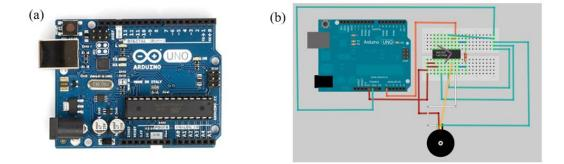
Fig. 6.2. Arduino Uno kit used to generate the code for load calculation (a) Arduino Uno circuit board ( $CourtesyofArduino^{(R)}$ ), (b) Arduino Uno breadboard connections[40]
