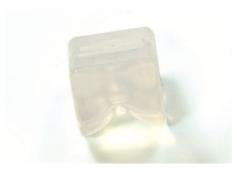
Fig. 5.9. 3D Printed Nose Bridge Part
