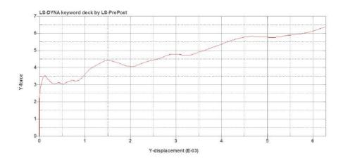
Fig. 4.2. Force-Deflection Curve. Slope=Spring constant=1.78 N/mm
