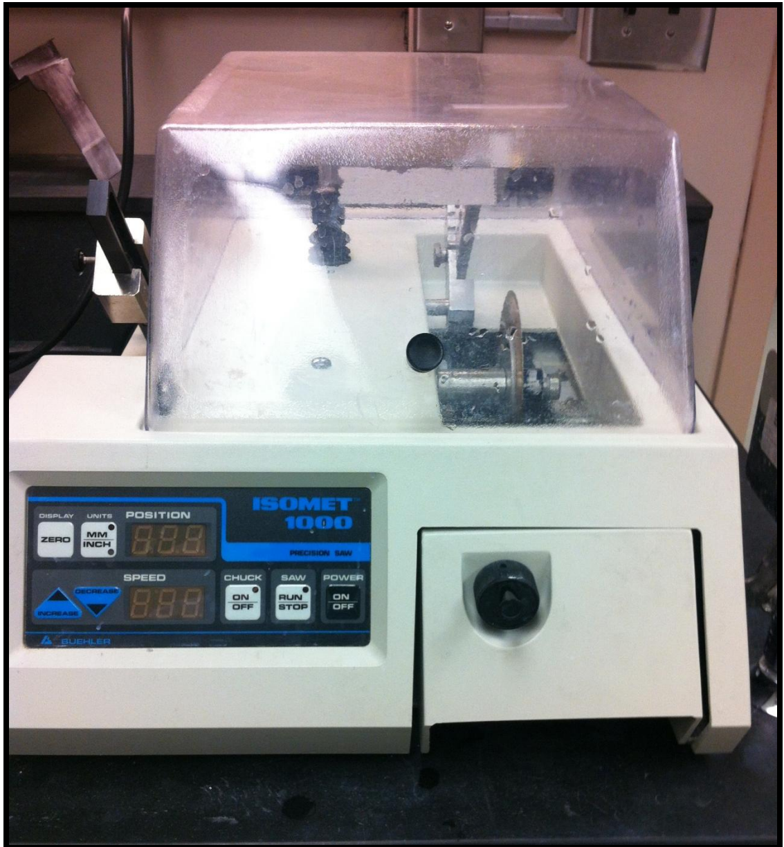
FIGURE 6. Low-speed cutting saw (Isomet 1000, Buehler, Lake Bluff, IL).
