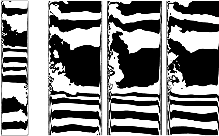
Figure 3: Instantaneous temperature field in a x_1 = cte plane. The isotherms are uniformly distributed from -0.5 to 0.5 . Left: general view of the cavity. Right: Time sequence of the top part of the cavity.
