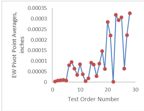
Figure 12: Horizontal Slippage of Bushing in the NS Direction (Direction of Table Motion) for Bushing 1.
