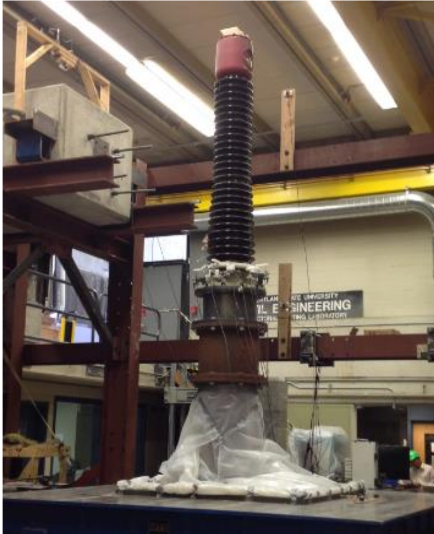
Figure 1: Full view of stiff setup for Bushing 1.
