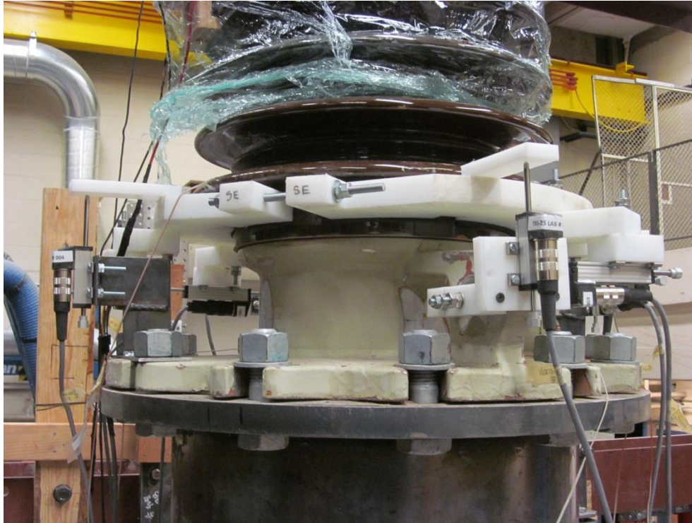
Figure 7: Photograph of LVDT's and instrumentation collar, southeast quadrant of bushing.
