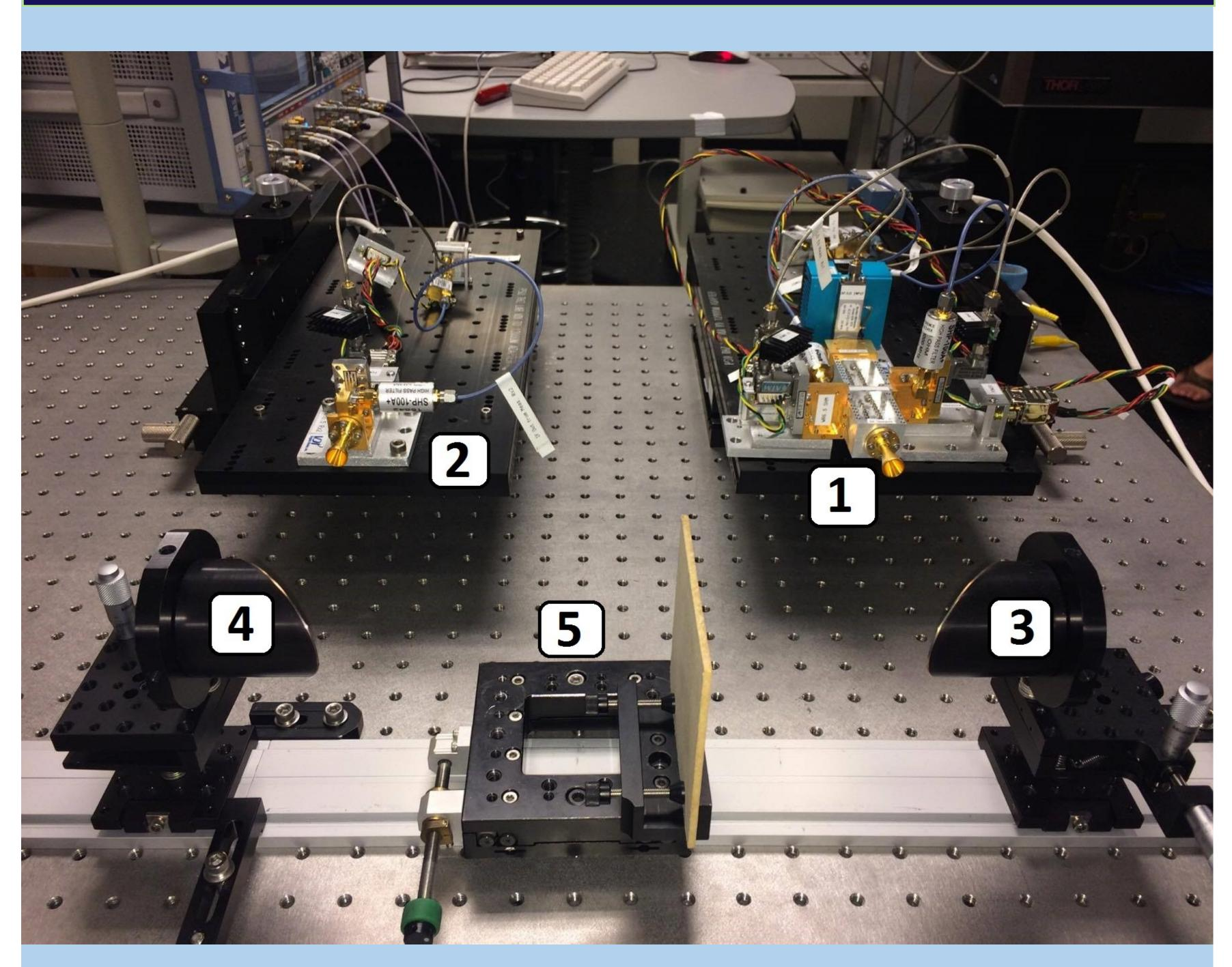
Quasi-optical measurement setup for WR-6.5 band: (1): Transceiver Module (2): Receiver Module (5):
