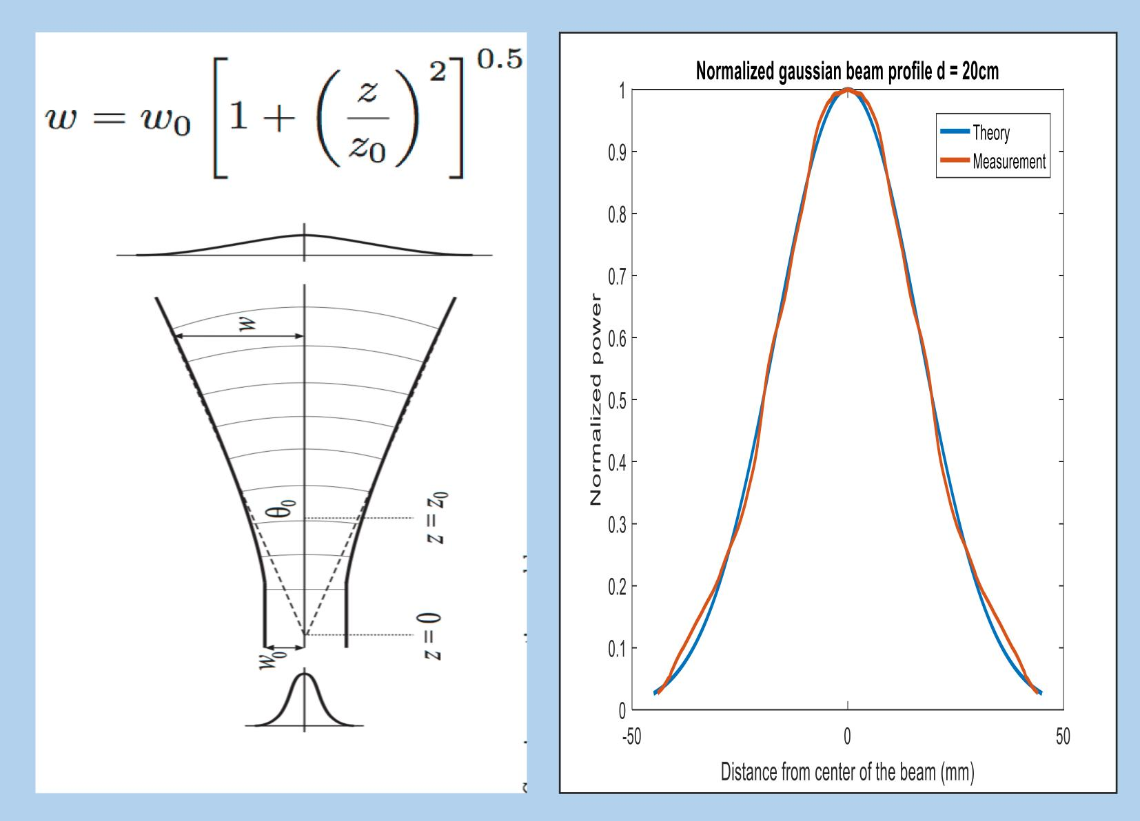
**THz optical path:** Two 90<sup> $^{0}$ </sup> off-axis parabolic mirrors are used to collimate and refocus the Gaussian beam.
