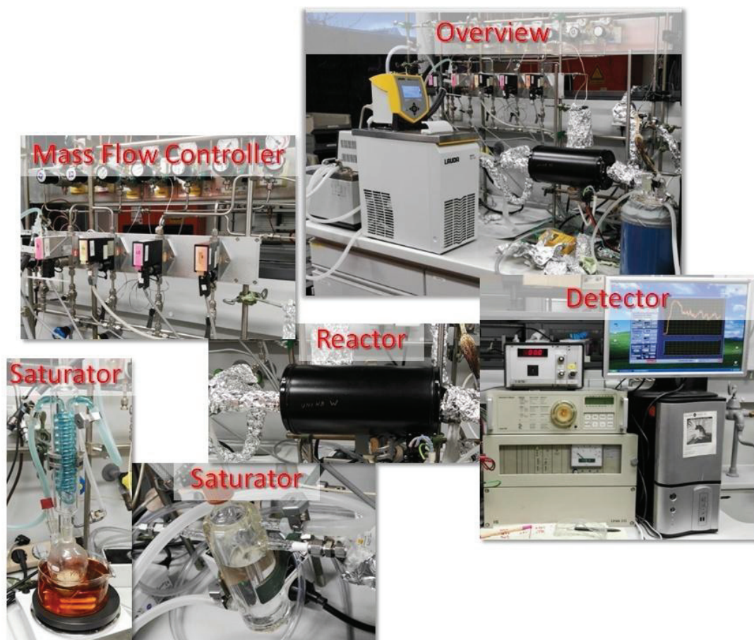
Figure 23. Experimental setup for measuring the catalytic performance of \text{MeO}_x/\text{npAu} . Flow and composition of gases were precisely controlled via mass flow controllers (upper left). The stream of gases was guided towards the reactor through a steel pipe, the outside of the pipe was wrapped with heating tape and covered with aluminum foil. For experiments using e.g. \text{H}_2\text{O} or methanol an additional He stream was guided through a saturator system to precisely adjust the content of the particular liquid in the gas phase.
