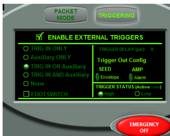
Figure A.5: Trigger Options on the Laser UI. LeNA is triggered via an auxiliary port. Therefore, the third option must be chosen. By default the trigger is in active low mode.
