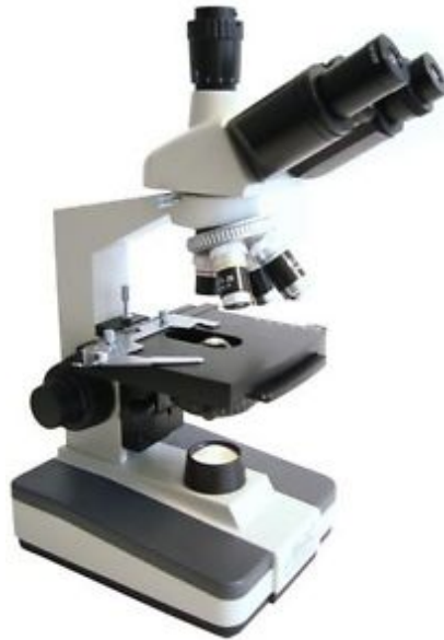
Figure 3.8: An image of a laboratory optical microscope. A halogen light bulb is situated at the base of the microscope that provides a broadband illumination to the sample. This is used to obtain transmission images in silicon by removing the neutral density filter. A camera is attached to the top to capture the infrared images.
