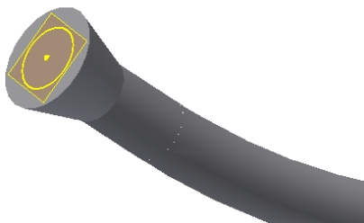
Figure 4.14: (a) A CAD design of 3DPOW, 270 \mu\text{m} in length and lenses on either of its ends. (b) The taper structure at the end of a 3DPOW of 9 \mu\text{m} diameter. (c) A lens fabricated at the end of the taper with a diameter of 15 \mu\text{m} .
