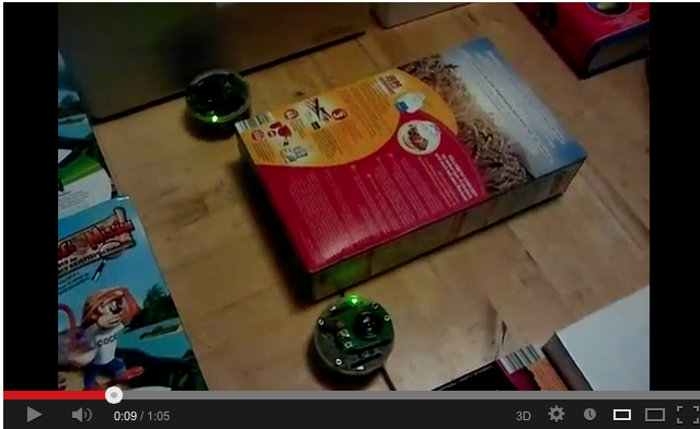
Figure 2: Screen shot of a demonstration of the final homework assignment. Each robot should explore the environment randomly, while it is avoiding obstacles (other robots and walls).
