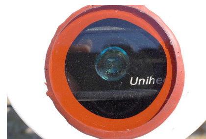
Figure 5.2: Aging of SQM plastic lens due to exposure to sunlight. Note the slightly yellowish color.
