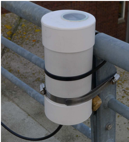
Figure 4.4: SQM-LE with manufacturer-supplied housing, mounted, pointing towards the zenith for night sky measurement [62].
