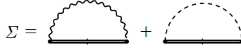
Figure 2.5.: Self energy diagrams with electron-phonon and electron-electron interaction that are included in the Eliashberg theory.
