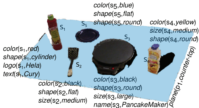
Figure 5.6: A kitchen scene in ROBOSHERLOCK with segmented regions of interest (clusters) and their logical annotations created by specialized perception routines.
