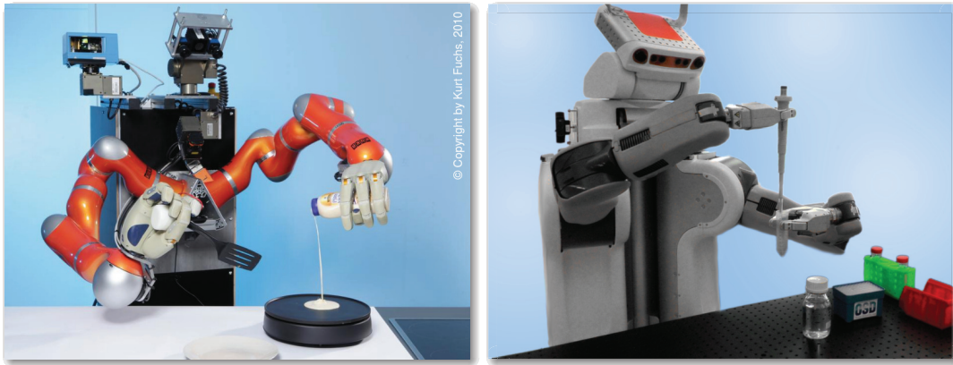
(a) The robot ‘TUM-Rosie’ preparing pancakes in a kitchen environment. (b) The robot ‘PR2’ performing a pipetting action in a chemical laboratory.
