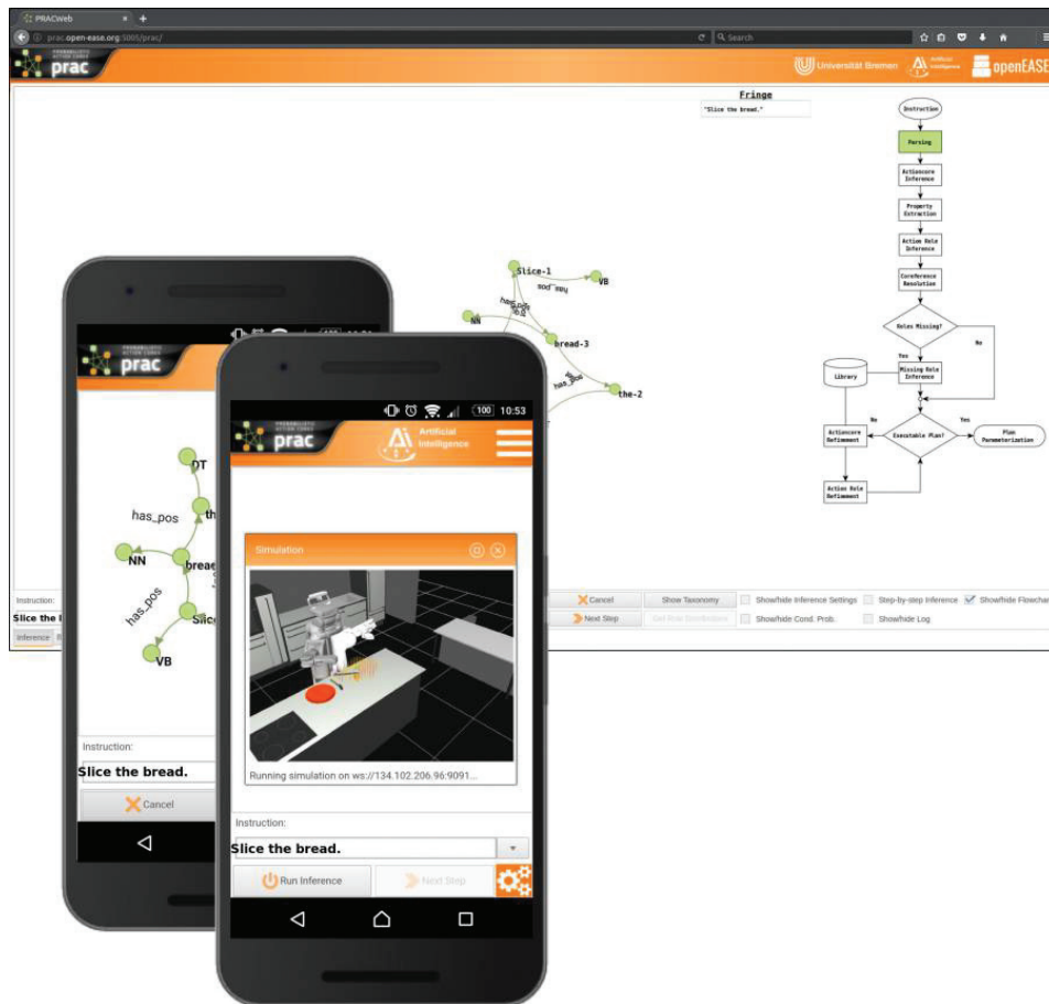
Figure 6.1: The browser-based web interface to PRAC on a desktop and a mobile client: the natural-language instruction “slice the bread” is transformed into the executable robot plan and executed in the web-based simulator. (courtesy of Mareike Picklum)
